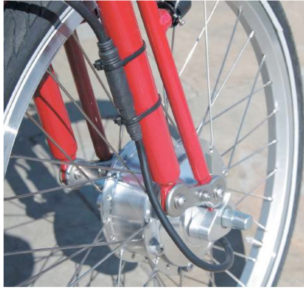
ABOVE: ARCC modify and strengthen the standard Moulton front dropouts to cope with the torque from the motor.
