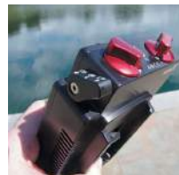
ABOVE: The Assist's main components are made from solid aluminium. The 'Dock' clamps securely to the bike's head tube. When the 'Pod' is clicked onto it, spring loaded contacts make all of the necessary electrical connections. Finally, a 36V Bosch power tool battery pack clicks securely onto the Pod.
