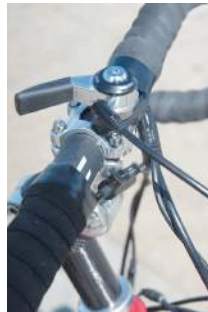
BELOW: With the rear hub gear changing gear automatically, there's just this single shifter for the front derailleur on the handlebars. Note also the brake cut-out sensors.
